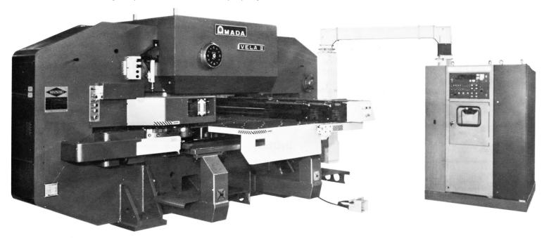
This 30 ton Vela II Amada Machine shapes and perforates our side panels with computer directed programming accurate to + .001".
